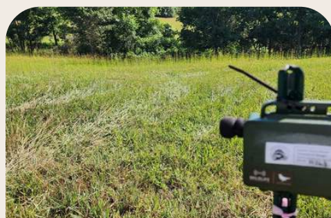
Autonomous Recording Unit (ARU) monitoring grassland birds
