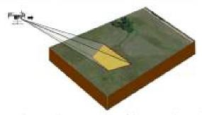
Camera: Representation of the approximate shape of the thermal coverage
