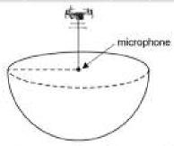
**Detector:** Representation of the approximate shape of the ultrasonic microphone coverage based on an assumed 20-meter detection range.
