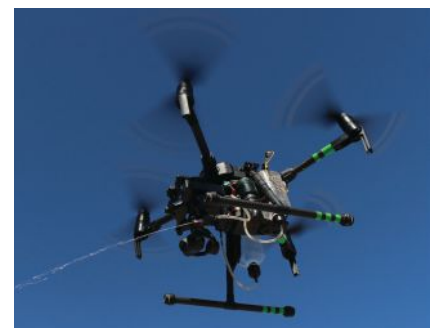
HardShell Labs uses drones for remote egg oiling to reduce the raven population.
