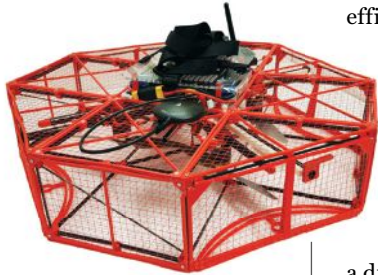
GearQuad has a protective cage inspired by the box turtle.
