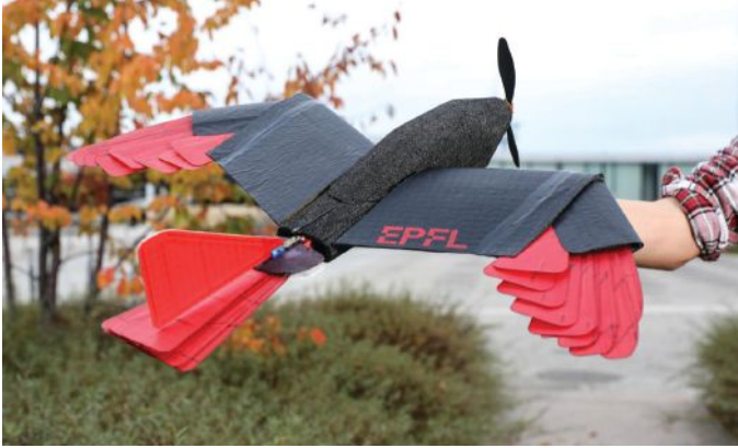
Inspired by the northern goshawk, the LisHawk possesses a morphing wing and tail with artificial feathers.
