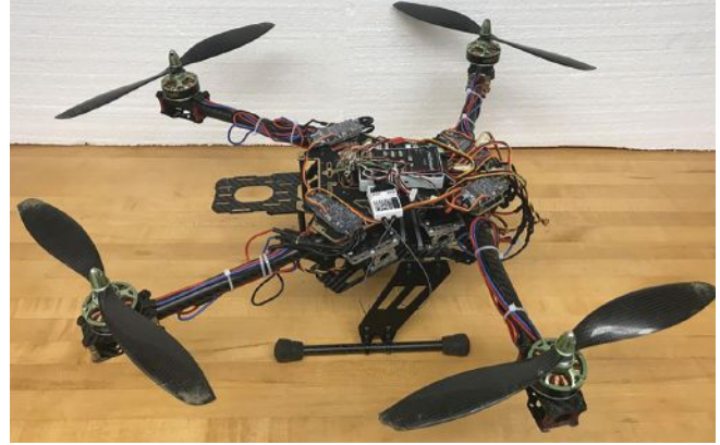
This insect-inspired drone from Purdue University can rotate its arms to alter its center of gravity and better balance its propellers' thrust.
