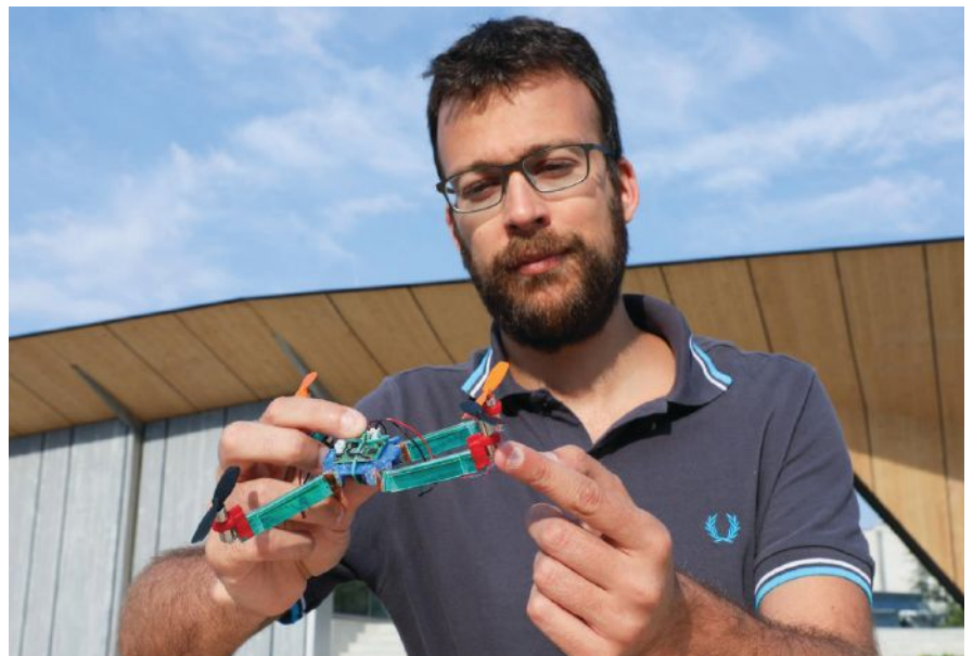
Swiss researcher Stefano Mintchev and his mini-drone. The drone's insect-wing inspired frame can deform upon impact and return to its original shape.
