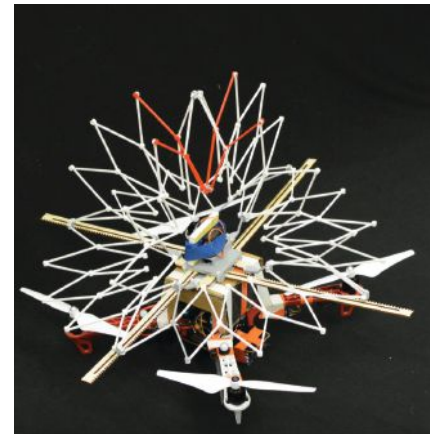
The PufferBot drone's adjustable protective cage is modeled on the pufferfish.
