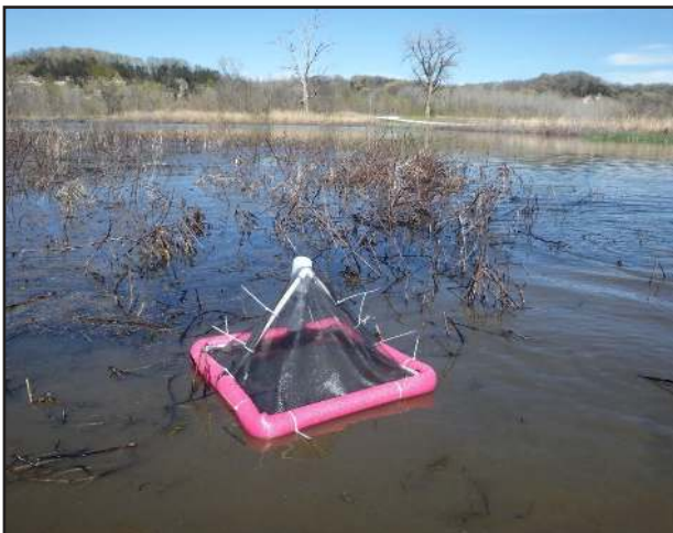
Floating aquatic emergent insect trap in study wetland used to measure available tree swallow forage. Photo by Kyle Kuechle.
