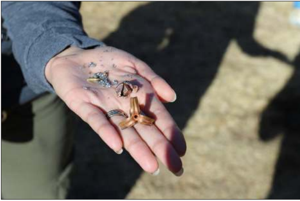
Lead bullet fragments and a non-lead expanded bullet collected from the water barrels.
