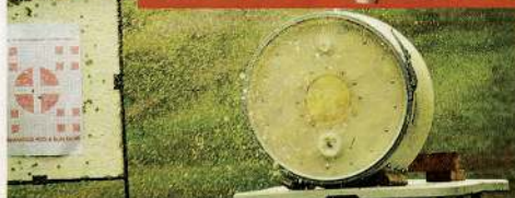
A lead bullet hits a barrel catch basin, where lead fragments can be collected by draining water.
