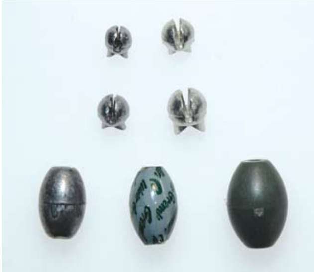
Figure 12. Relative sizes of sinkers manufactured from different materials. Top row: 0.1 oz lead and tin split shot. 2nd row: 0.2 oz lead and tin split shot. 3rd row: 0.8 oz lead, bismuth, and plastic/iron composite egg sinkers. (courtesy of Water Gremlin. Photograph by T. Lawrence, Great Lakes Fishery Commission)
