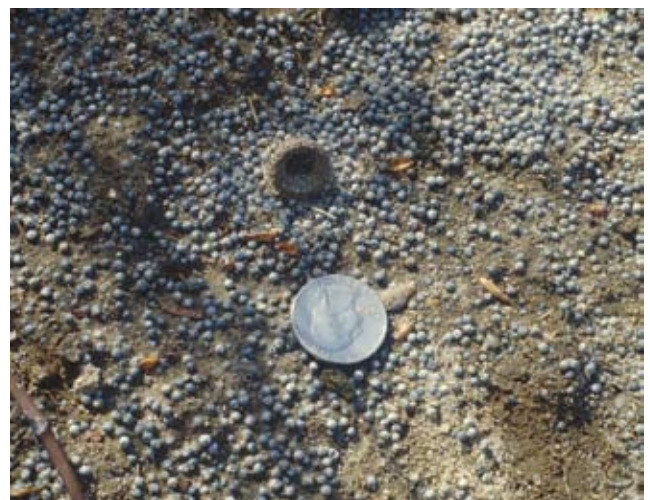
Figure 3. Lead shot with white oxide or carbonate coatings on surface in the fall zone at the Broadkilm Sportsman's Club (24 mm coin for scale). (courtesy of Daniel J. Soeder, U.S. Geological Survey).
